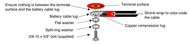
Figure 2-12 Battery Cable Connection
