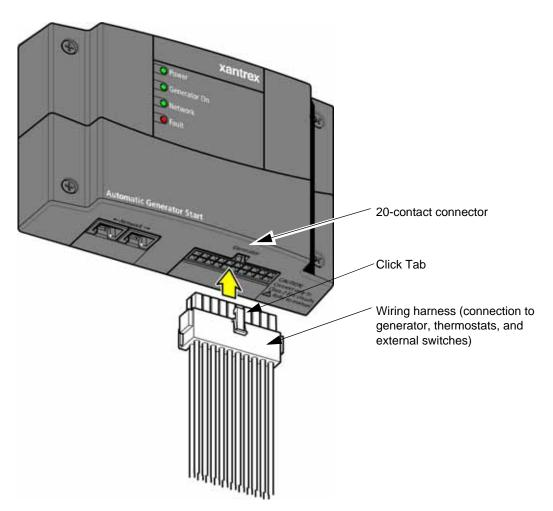
Figure 5-11 XW Automatic Generator Start External Connections
