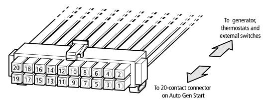
Figure 5-9 XW Automatic Generator Start Wiring Harness
