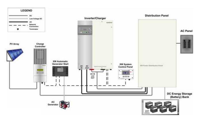
Figure 3-1 Network-Managed Power System
