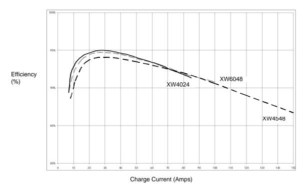
Figure A-6 Charging Efficiency (Typical)
