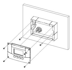
Figure 5-6 Surface Mounting the XW System Control Panel
