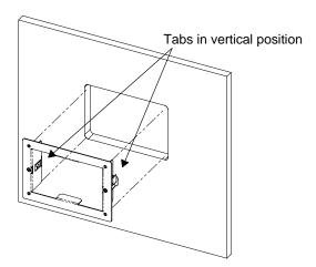
Figure 5-2 Inserting the Mounting Plate
