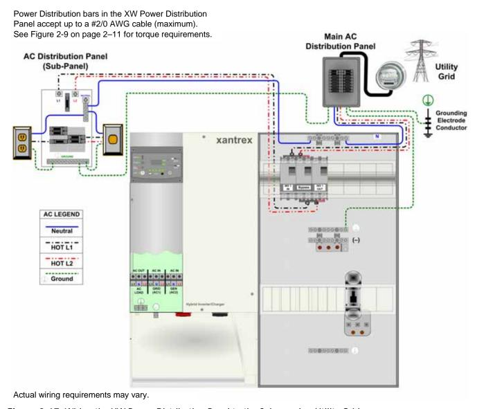
Figure 2-17 Wiring the XW Power Distribution Panel to the Sub-panel or Utility Grid
