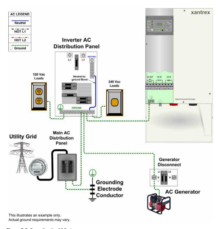
Figure C-3 Grounding the AC System
