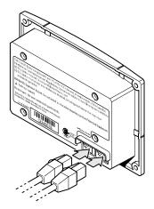
Figure 5-4 Connecting the Network Cables
