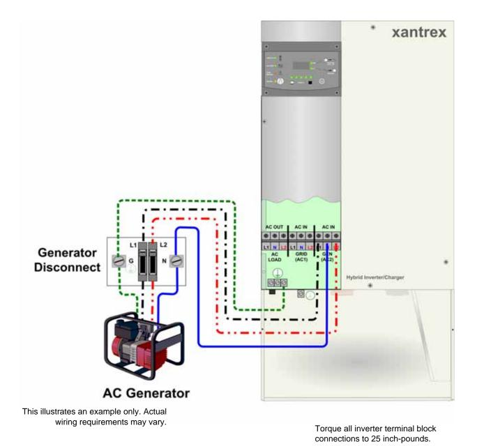
Figure C-5 Generator Wiring directly to the Inverter
