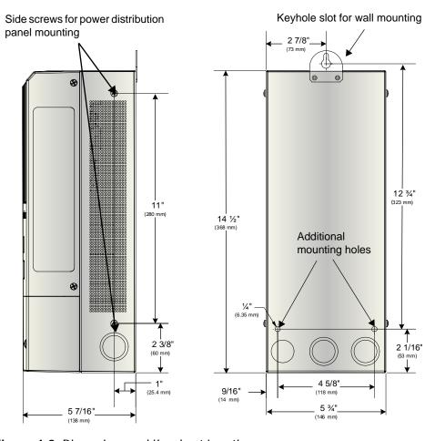
Figure 4-3 Dimensions and Knockout Locations
