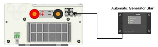
Figure 5-7 Connecting the AGS Communications Cable to the XW Series
