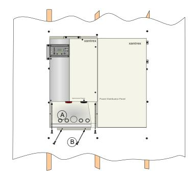
Attach the back panel of the XW Conduit Box to the bottom of the inverter with two screws through the keyhole slots under the back panel top and the corresponding holes in the bottom of the inverter (A). Secure the bottom edge of the back panel to the wall using two screws (B).
