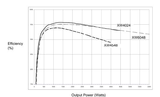
Figure A-5 Inverting Efficiency (Typical)
