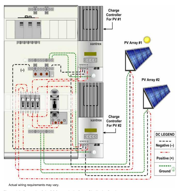
Figure 4-9 Connecting Solar DC Sources in the Power Distribution Panel
