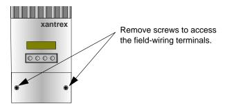
Figure 4-2 Removing the Wiring Compartment Cover
