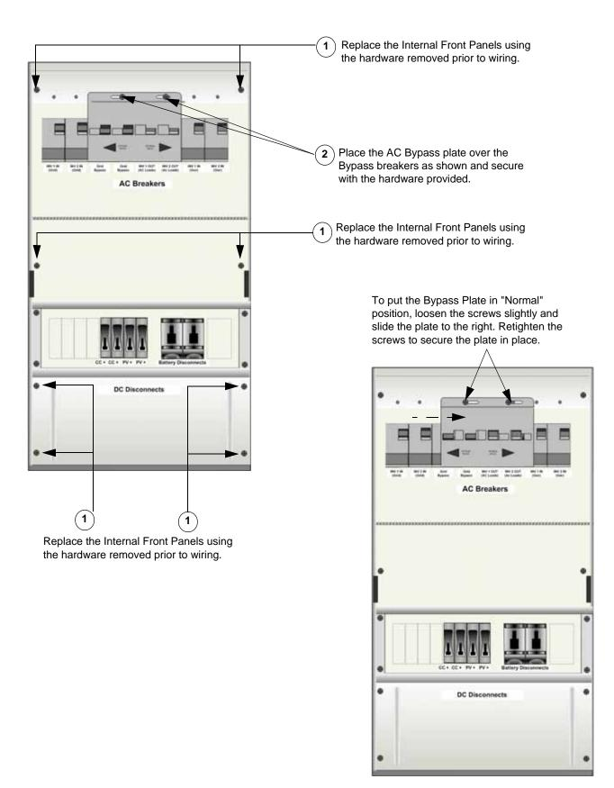
Figure 2-30 Installing the Front Internal Panels and the AC Bypass Plate
