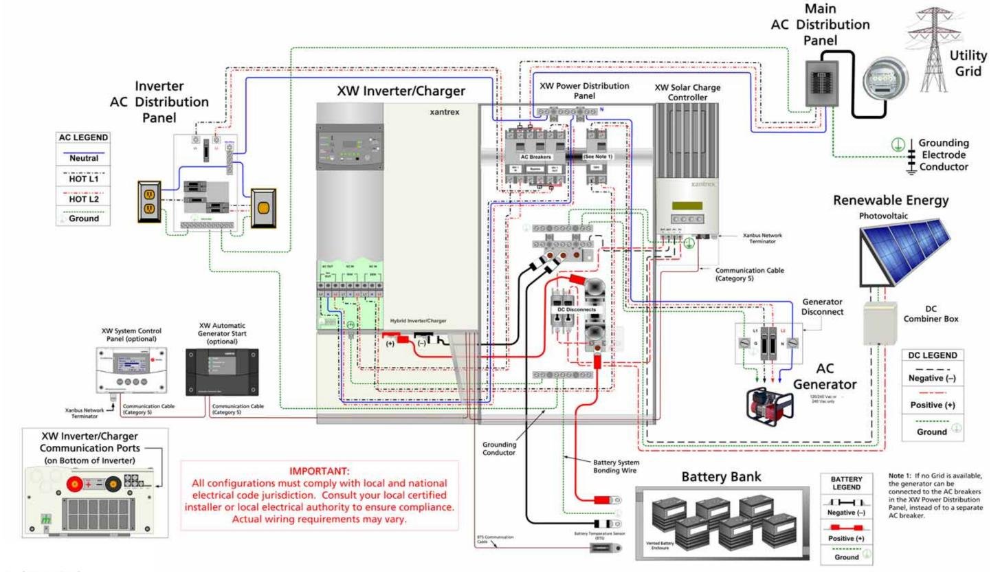
Figure B-3 Single-Inverter System Renewable Energy (Solar)
