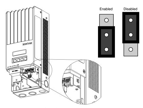
Figure 4-7 PV Negative Ground Jumper Location
