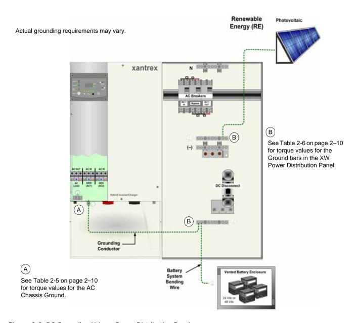
Figure 2-9 DC Grounding Using a Power Distribution Panel
