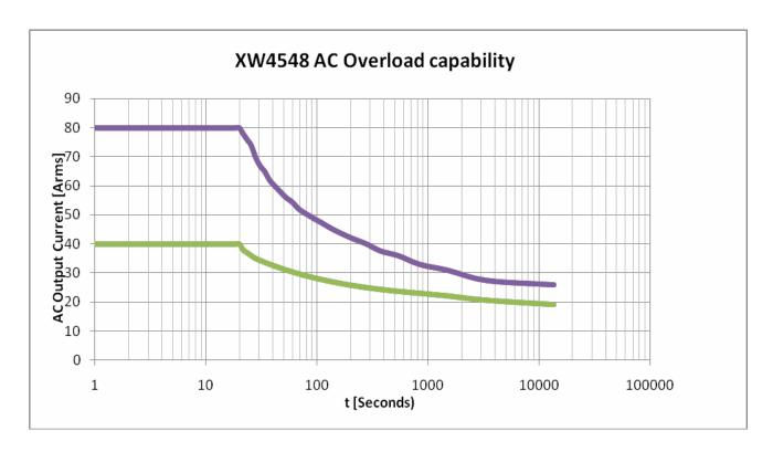
Figure A-2 XW Series AC Overload Capability
