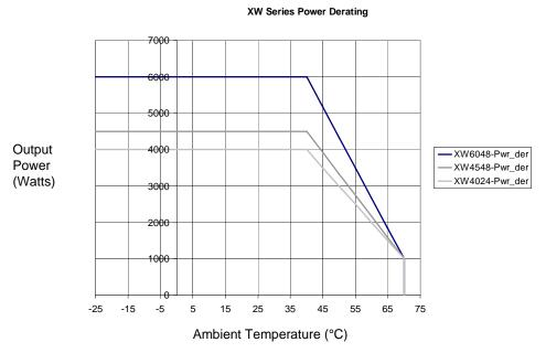
Figure A-4 Output Power Versus Ambient Temperature
