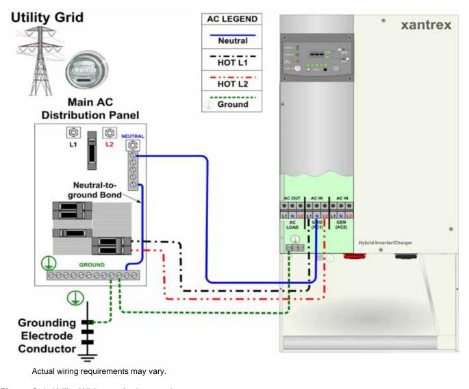
Figure C-6 Utility Wiring to the Inverter Input
