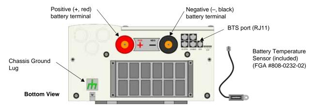
Figure 2-11 XW Inverter/Charger DC Connections
