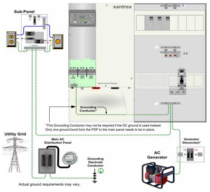
In an off-grid installation (i.e., where no utility grid is available), the generator can be connected to the breakers provided in the XW Power Distribution Panel. No additional breaker is required.
