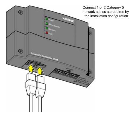
Figure 5-12 Connecting the SCP
