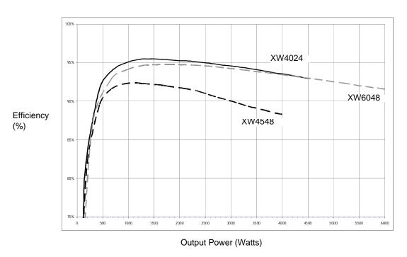
Figure A-8 Grid-tie Sell Mode Efficiency (Typical)
