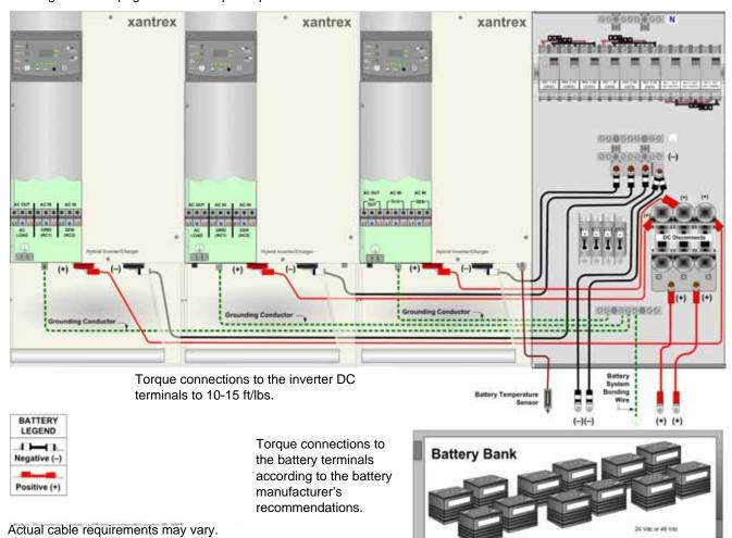
Figure 2-31 DC Connections for a Triple-Inverter System
