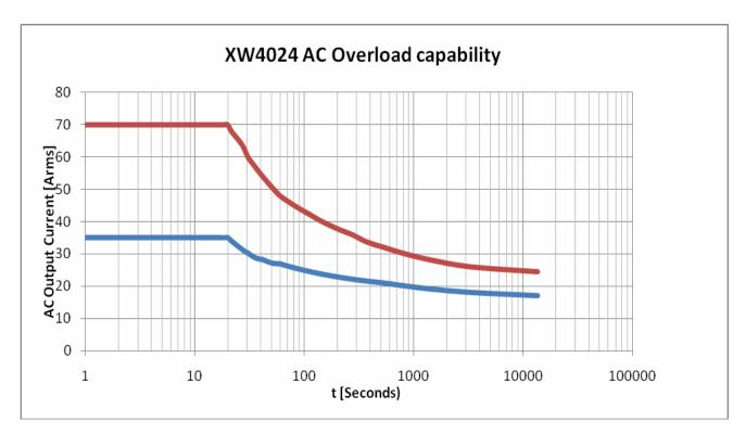
Figure A-3 XW Series AC Overload Capability
