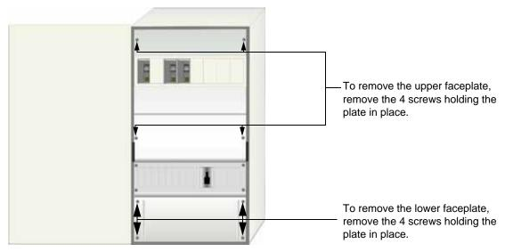
Figure 2-2 Removing the Internal Faceplates on the Power Distribution Panel
