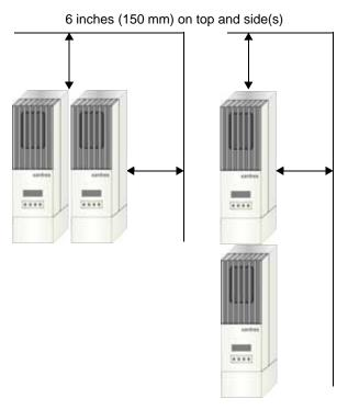
Figure 4-1 Minimum Clearance Requirements
