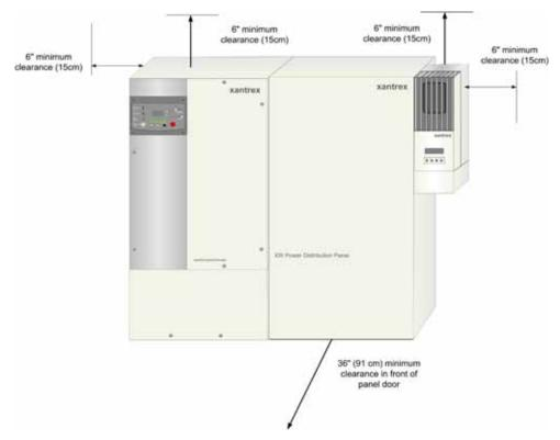
Figure 2-3 Clearance Requirements
