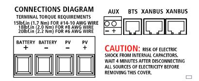
Figure 4-8 DC Connection Terminals
