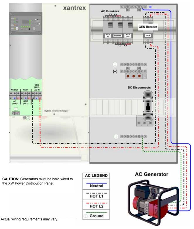
Figure 2-19 Generator Wiring Using a XW Power Distribution Panel (On Grid)
