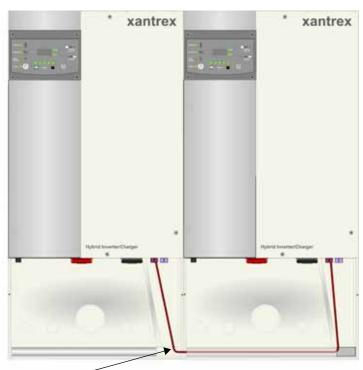
Route the cable as shown. Route any additional communication cables through the raceways. Replace the wiring raceways, ensuring not to pinch the cables. Secure the raceways to the XW Conduit Box with the screw that was removed earlier.
