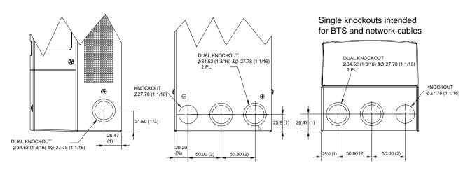
Figure 4-4 Knockout Dimensions
