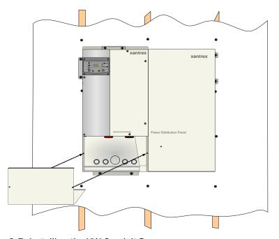
Attach the front panel of the XW Conduit Box by sliding the bottom lip of the front panel over the lower edge of the back panel. Align the two holes in the front panel with the two holes in the back panel. Use the two #10-32 screws provided to secure the front panel to the back panel.
