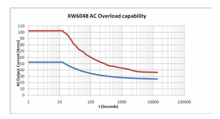
Figure A-1 XW Series AC Overload Capability
