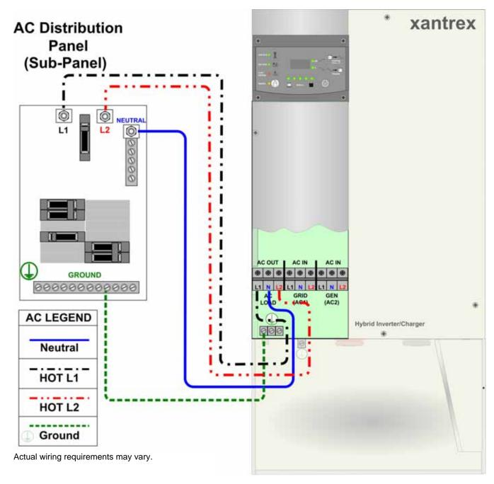
Figure C-4 AC Output Wiring to the Inverter AC Distribution Panel
