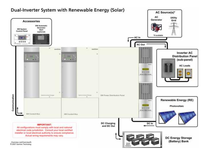
Figure 1-1 XW Power System Installation Diagram Example
