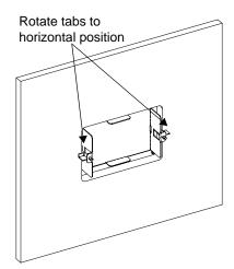
Figure 5-3 Securing the Mounting Plate
