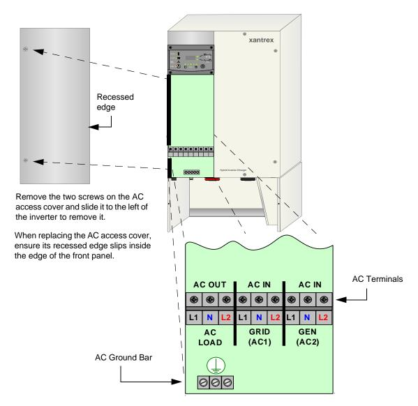
Figure 2-15 AC Terminal Block
