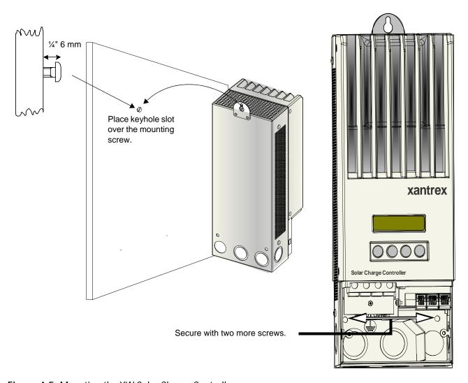
Figure 4-5 Mounting the XW Solar Charge Controller
