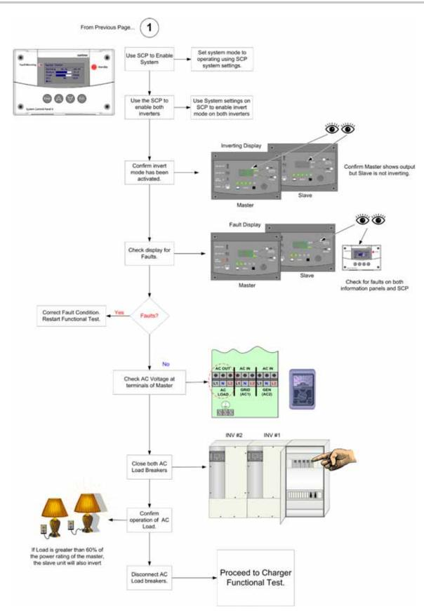
Figure 2-37 Functional Test for Multiple Inverters - Page 2 of 2
