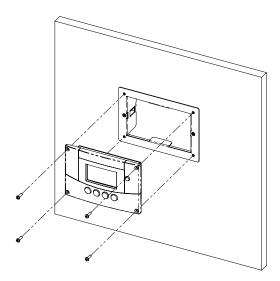
Figure 5-5 Securing the XW System Control Panel
